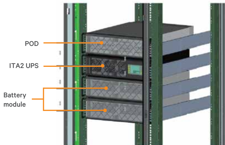
Isometric view of Liebert® ITA2 UPS installed in a rack-mounted alignment along with POD and Battery modules
